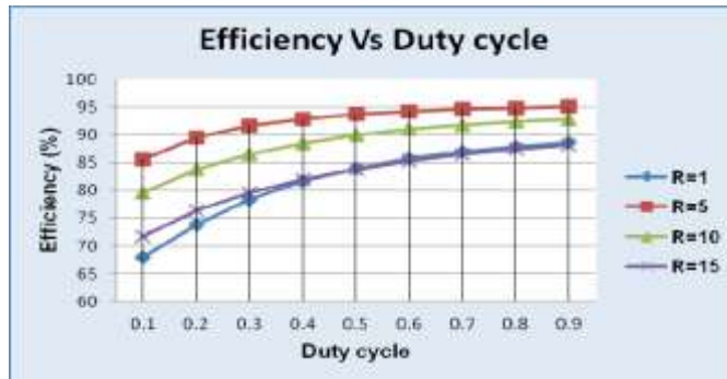
Fig. 7. Efficiency Vs Duty Cycle for different pan resistance
