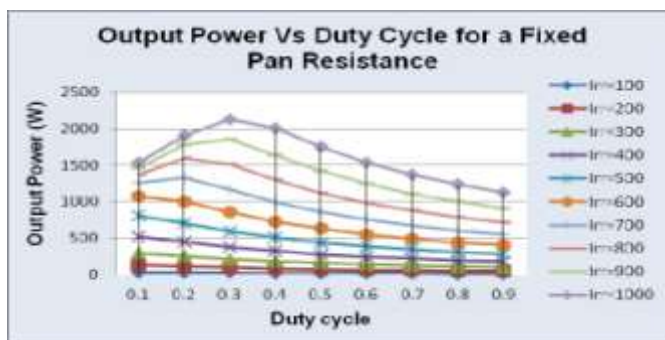
Fig. 10. Output Power Vs. Duty Cycle at different solar irradiation levels
